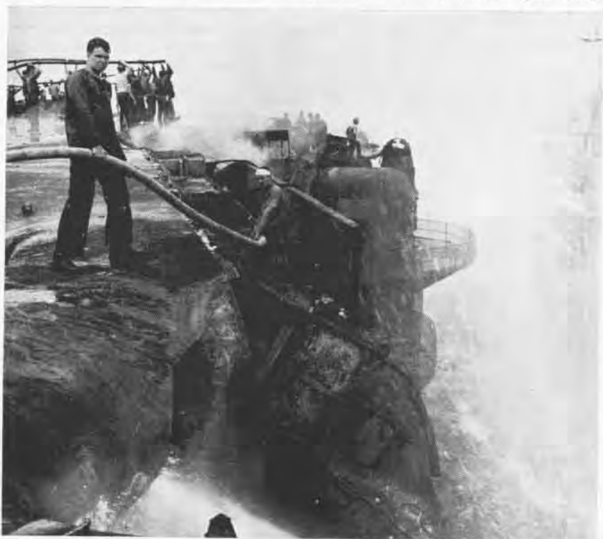
PROTECTED by OBA's, Forrestal crewmen brave smoke to fight below-decks fires through holes blasted in the flight deck (above). As destroyer maneuvers alongside and sends streams of water over (below), other Forrestal men battle interior fires from accesses in nearly destroyed flight deck catwalk. Hump in rear is one of the attack carrier's five-inch gun mounts.
