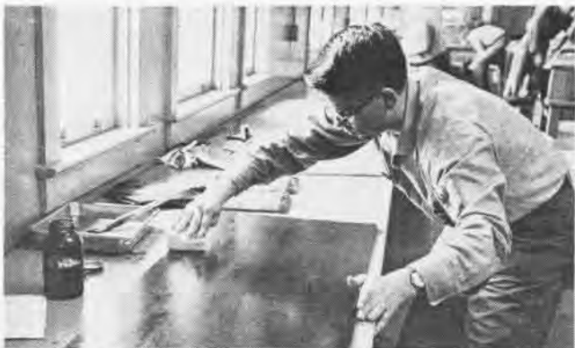
IN PREPARING a masonite board for cementing, Keller takes the final steps toward producing an aerial map of the entire target area.
