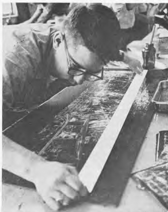
AFTER ADJUSTING image points and cementing photos to the board, PH3 Keller puts on final touch: the border to set off his work.
