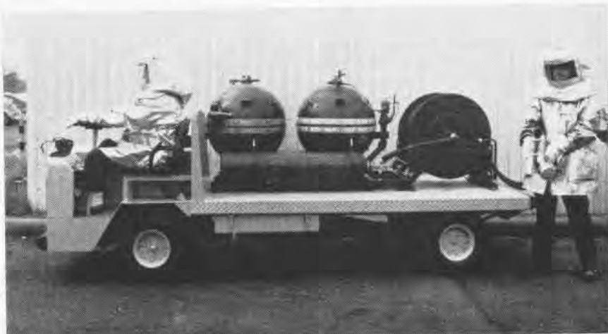
THE SPHERES ON A LINE SERVICE TRUCK CARRY LIGHT WATER AND PURPLE-K-POWDER
